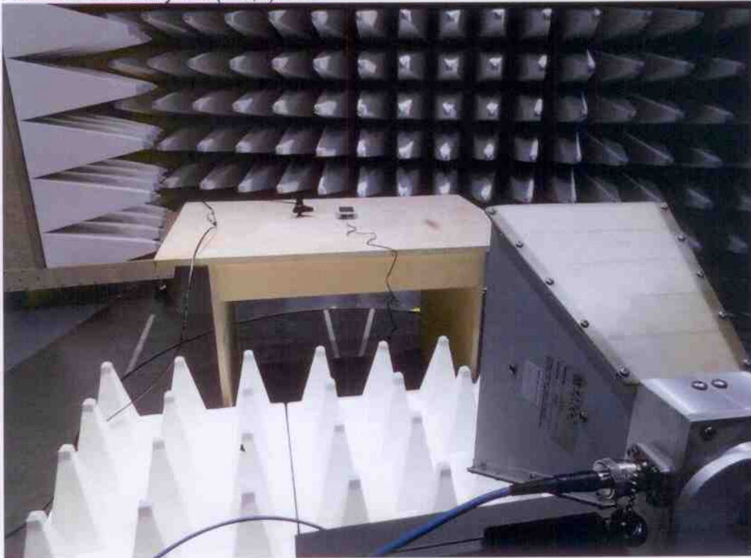
Radiated immunity test(1-2,7)GHz
