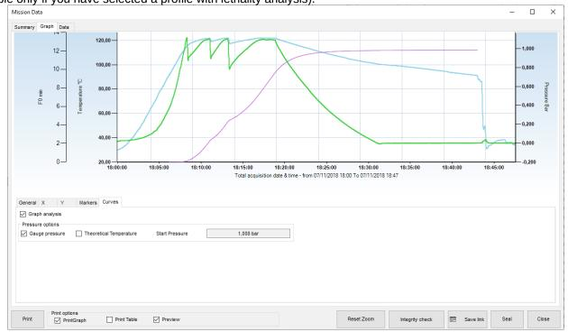
Pressure curve options: gauge pressure and theoretical temperature
