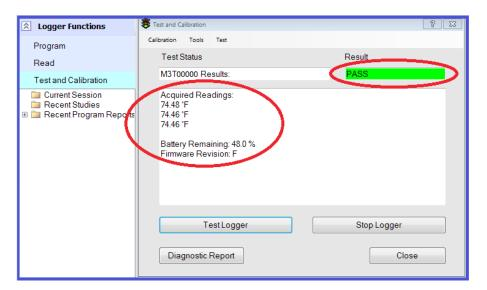
**NOTE:** The Test function will not affect Programming or Reading. However, if you have unread data currently residing in a logger's memory, the Test function will override and erase it. Please Read the logger first if unread data is present. Read instructions are on Page 8 of this guide.
