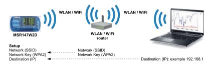
For this option you do not require any additional hardware, as it uses the existing network infrastructure. There is no internet access needed, as the measuring data is sent to a local application.
