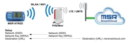
In this option an additional WiFi network and internet access using a mobile phone connection are provided — e.g. through a Fritx!Box. A suitable Fritz!Box as well as a SIM card that can be used in many countries is available from MSR Electronics GmbH upon request. The configuration instruction for the Fritz!Box is available in the support area on www.cik-solutions.com/en-msr-support
