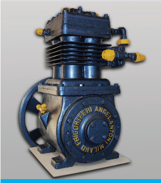
Double stage refrigeration compressor patented in 1949
