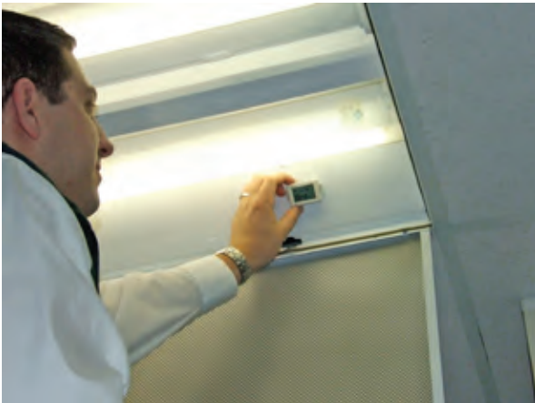
Mounting of a data logger can be quick and easy with built in rare earth magnets.
