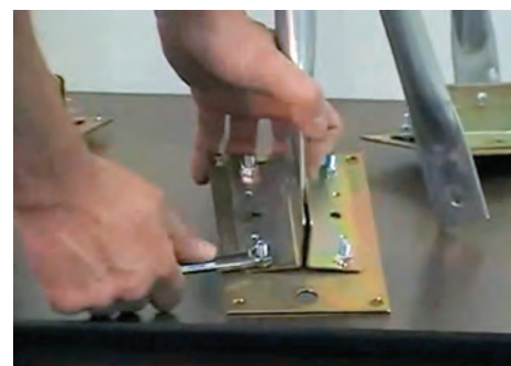
Partial assembly of a weather station indoors can help reduce the loss of small parts in the field.
