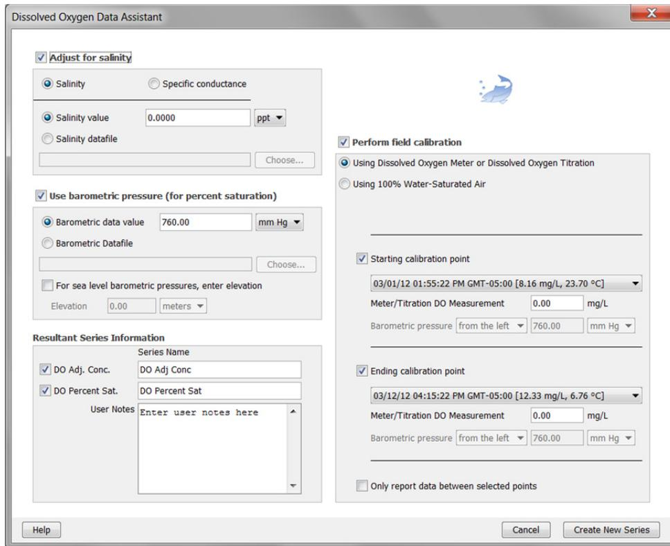
4. **Adjust for salinity.** If you deployed the logger in saltwater, you must adjust for salinity to get either a DO concentration or percent saturation. To do this, select the “Adjust for Salinity” checkbox (you will also need to select the checkboxes under Resultant Series Information for the series you would like). Select whether the series should be adjusted based on salinity or specific conductance.
