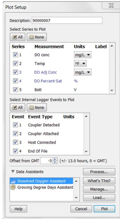
10. Click the Plot button to plot the data. After the plot is displayed, you may apply minimum, maximum, and average filters to the scaled series as you would for any sensor data series in HOBOWare Pro.
