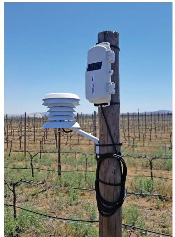
Look for smaller transmitters that have integrated solar panels for easy deployment.
