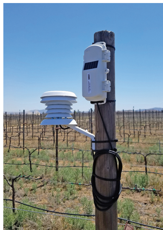
Look for wireless sensors that are small and that have integrated solar panels for easy deployment.
